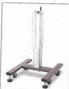
Totally-enclosed telescoping stand has a load capacity up to 1,000 lb. The stand column is made from clear anodized aluminum with a steel weldment base and comes with holes for easily mounting equipment. An adjusting screw with a hand crank enables height adjustments
